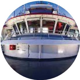
**Superstructure:** The non-sacrificial barrier created by Coval Marine blocks moisture, air, and chlorides to effectively prevent topside degradation due to salt-spray, galvanic corrosion, cathodic disbondment, and UV oxidation.
