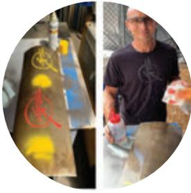
**Anti-graffiti:** Paint, markers, and stains of all forms do not penetrate the coating and are easily removed with a mild solvent such as Isopropyl alcohol. This results in less maintenance and chemical costs, and swift removal discourages taggers from repeat offenses.
